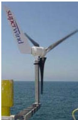
A wind turbine (wind generator) is a system that converts the kinetic energy of the wind into electricity. The principal of operation is similar to a hydroelectric generator. The main difference is the medium that is being utilized, running water for the first and blowing wind for the latter.
