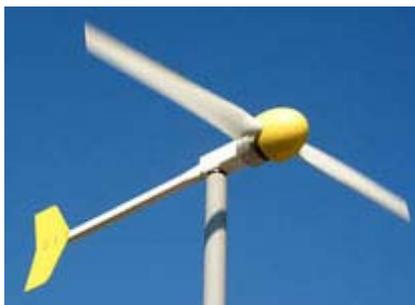
Experimentation has shown that the best design philosophy, with the objective of producing the maximum possible power for the lowest cost and at the same time at the highest reliability, is that of a horizontal upwind, 2 or 3 blades lifting style airfoil
